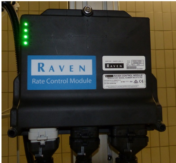
Fig. 3: PWM control module on sprayer boom.
